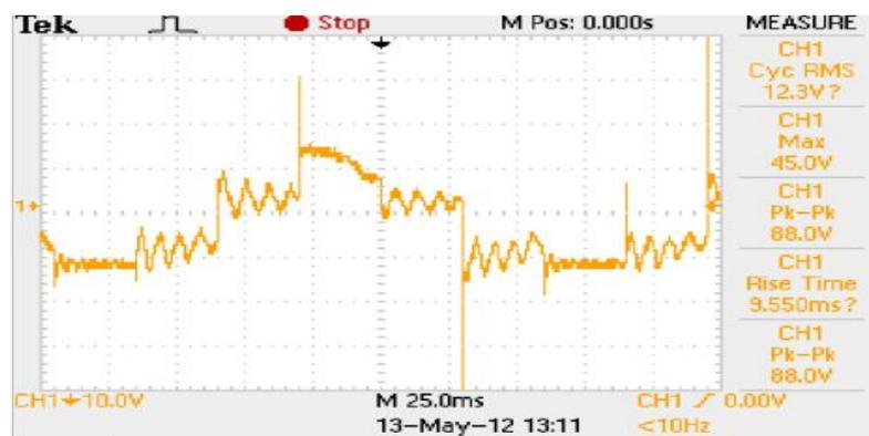
Fig.6 Output of power circuit ( $V_{R \text{ phase-phase}}$ ) of conventional method
