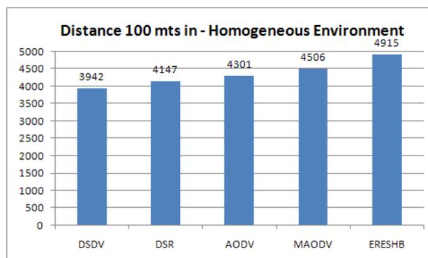
Fig.2. Distance Vs Throughput in homogeneous environment
