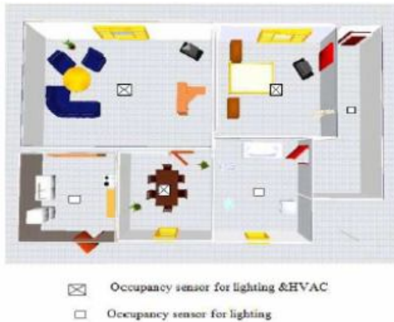
Fig. 4 : Layout of apartment indicating the distribution of sensors used (Sweet Home 3D software)
