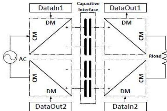
Figure 7: Simplified Power and Data Transfer Block Diagram
