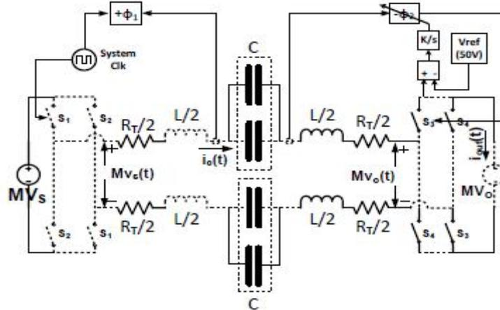
Figure 9: Series Resonant Converter with Phase Feedback
