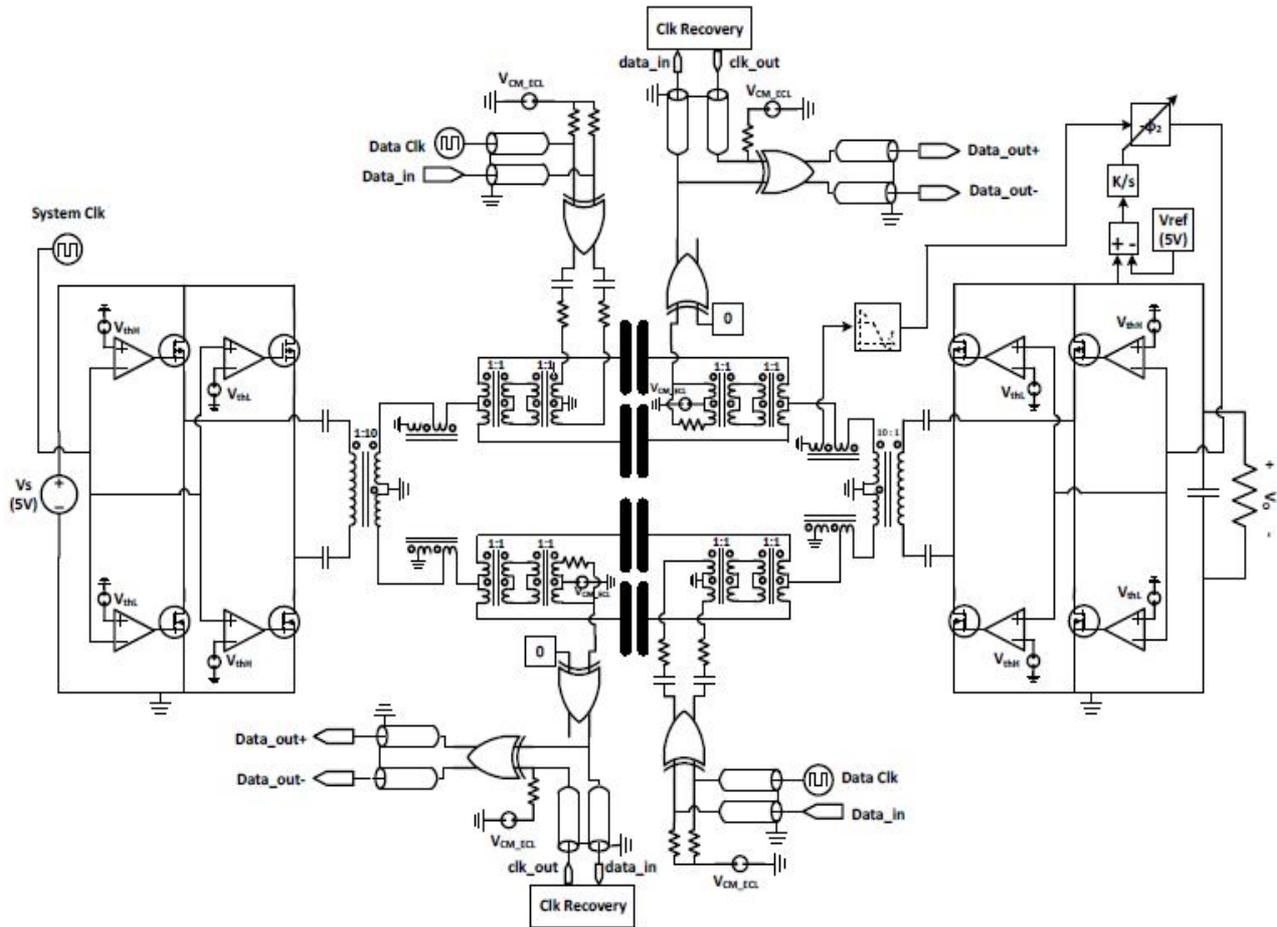
Figure 8: Detailed Capacitive Power and Data Transfer
