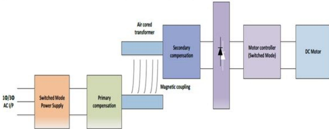
Figure 1: An IPT system for powering an EV
