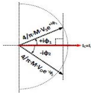
Figure 10: Series Resonant Converter with Phase Feedback
