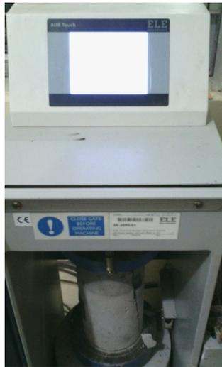
Fig. 4 – Testing Concrete Pressure by using ELE machine
