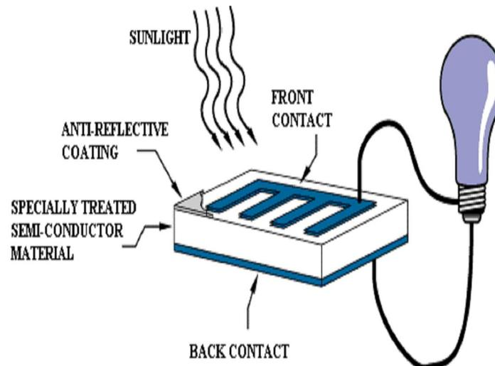
Fig. 2 Photovoltaic Process
