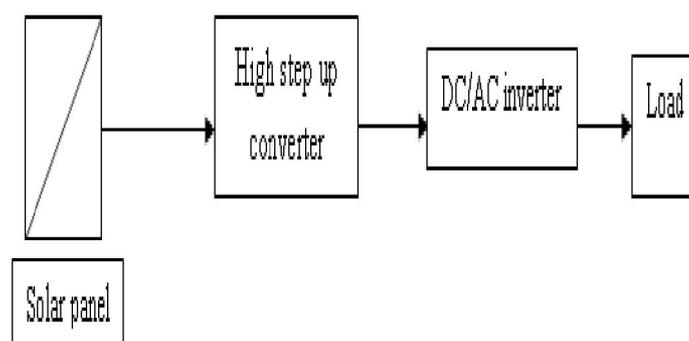
Fig. 1 Block diagram of photovoltaic system
