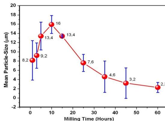
Fig.2. the mean particle size of SrCO<sub>3</sub> and TiO<sub>2</sub> mixture as function of milling time
