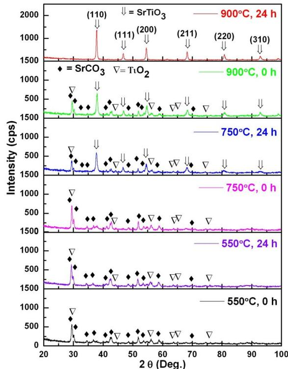
Fig.5. X-ray diffraction profile of SrCO<sub>3</sub> and TiO<sub>2</sub> mixture after annealing up to 900°C.
