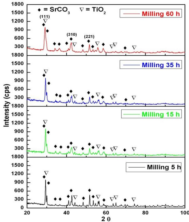
Fig.3. X-ray diffraction patterns of SrCO<sub>3</sub> and TiO<sub>2</sub> mixture up to 60 hours of milling
