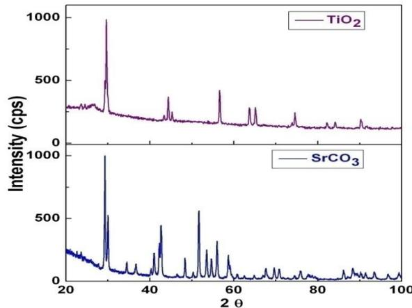
Fig.1. X-ray diffraction patterns of SrCO<sub>3</sub> and TiO<sub>2</sub> precursors
