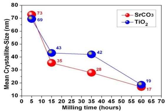
Fig.4. The mean crystallite size of SrCO<sub>3</sub> and TiO<sub>2</sub> mixture up to 60 hours of milling
