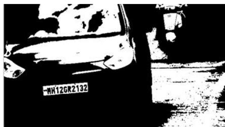
Fig 6:-Image after opening operation
