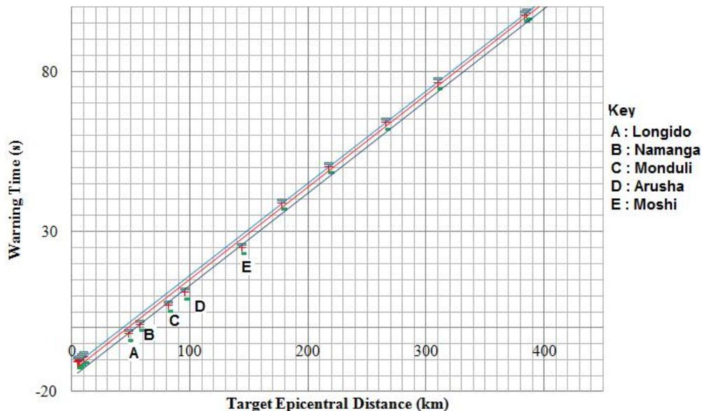
Fig 7: Warning times with new stations at varying station trigger thresholds. Green (bottom) line represents warning times with five trigger thresholds, Red (middle) line represents warning times with three station trigger threshold, and Blue (upper) line represents warning times with one station trigger threshold.
