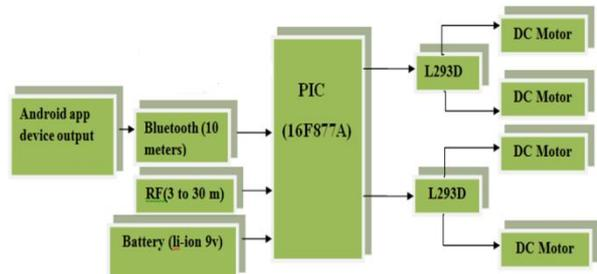
Fig 1.B receiver section
