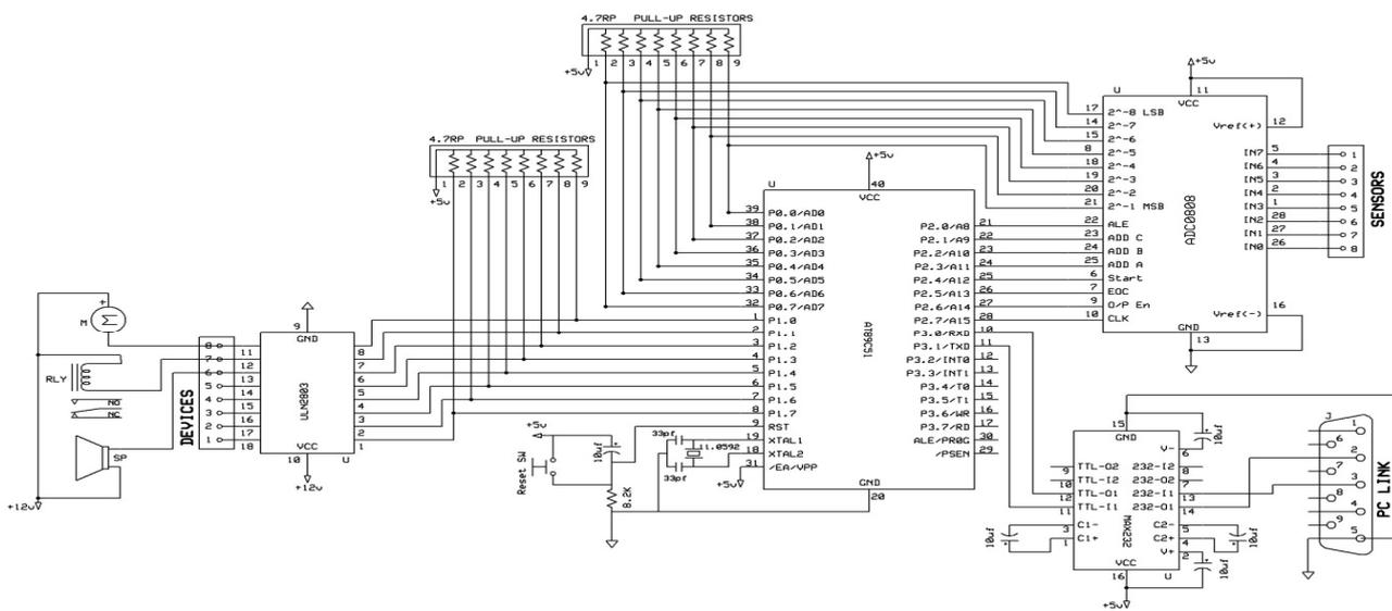
Fig.5: Intelligent Drip Irrigation System - Circuit Diagram
