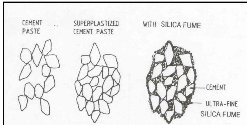
Fig.5: Dense microstructure of concrete due to use of micro silica
