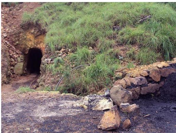
Fig. 3: Extraction of coal by ‘Rat-hole’ mining
