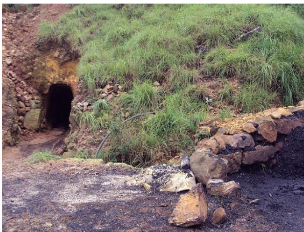
Fig. 3: Extraction of coal by ‘Rat-hole’ mining
