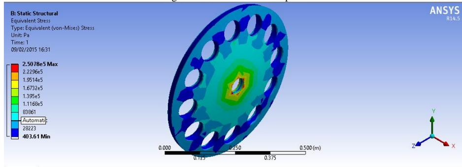
Fig. 12 Stresses in base plate
