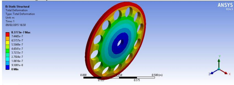
Fig. 11 Deformation of base plate
