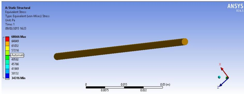
Fig. 6 Stresses in stacker rod
