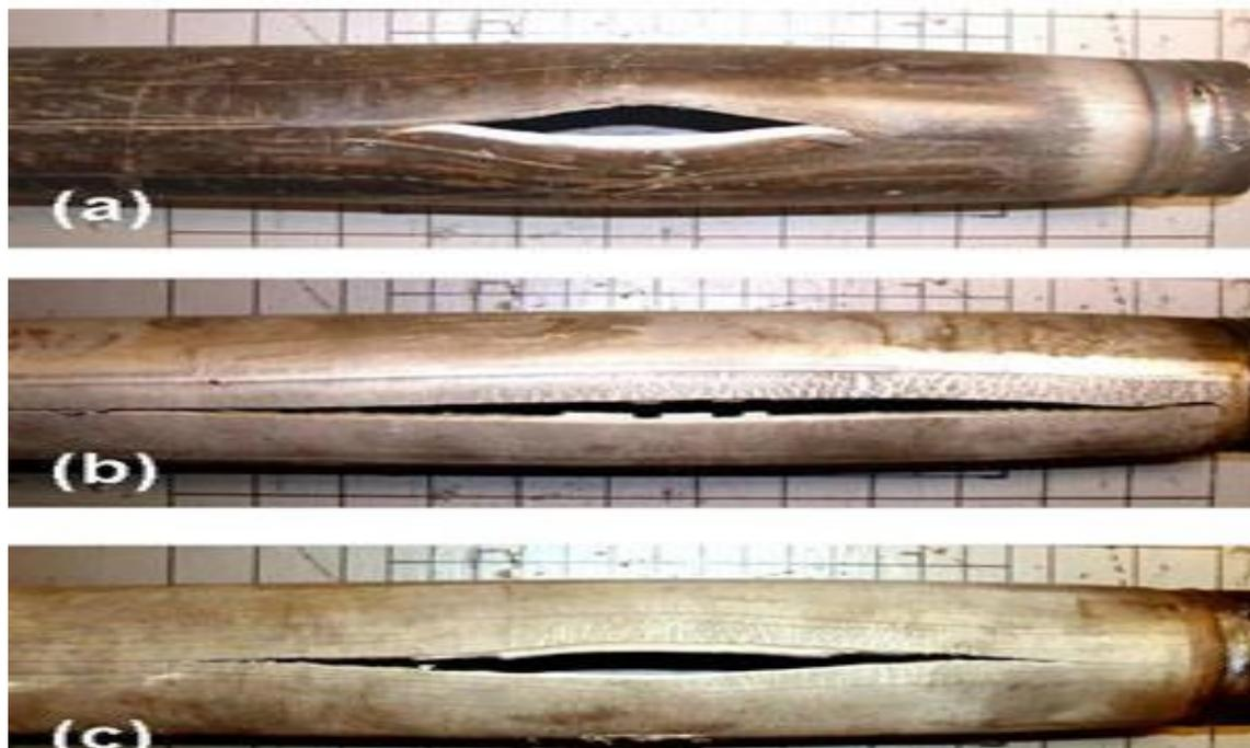
Fig. 4.2 Some of the Damaged Super Heater Tubes.
