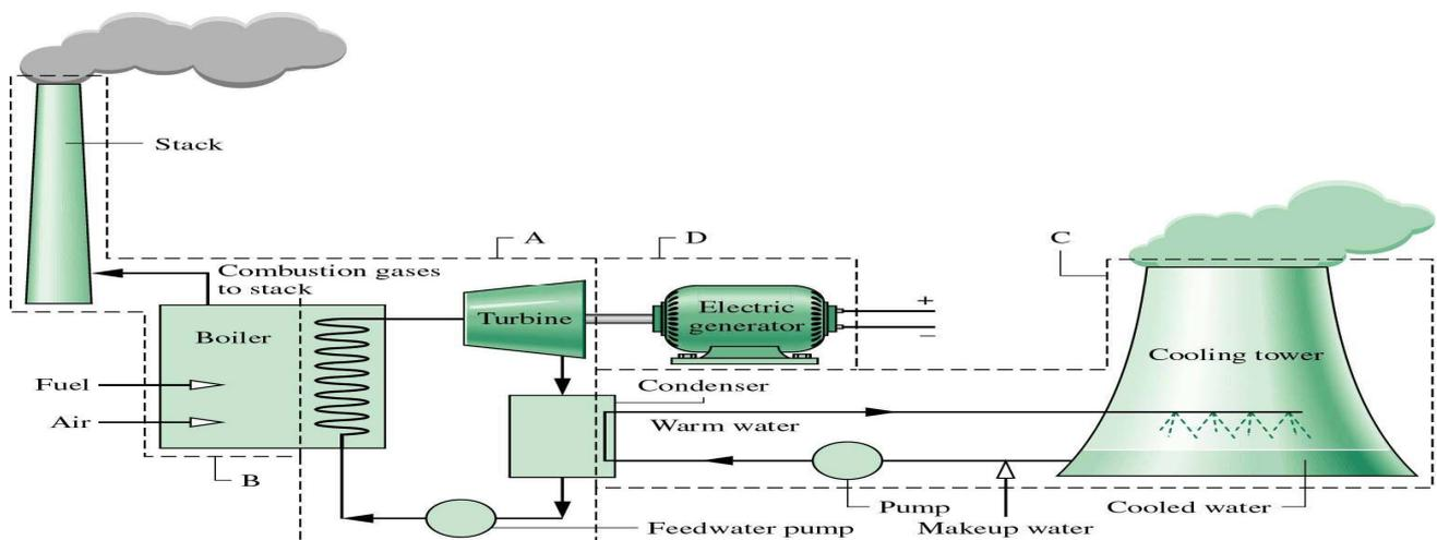
(Fig. 1.1) Schematic Diagram of Thermal Power Plant
