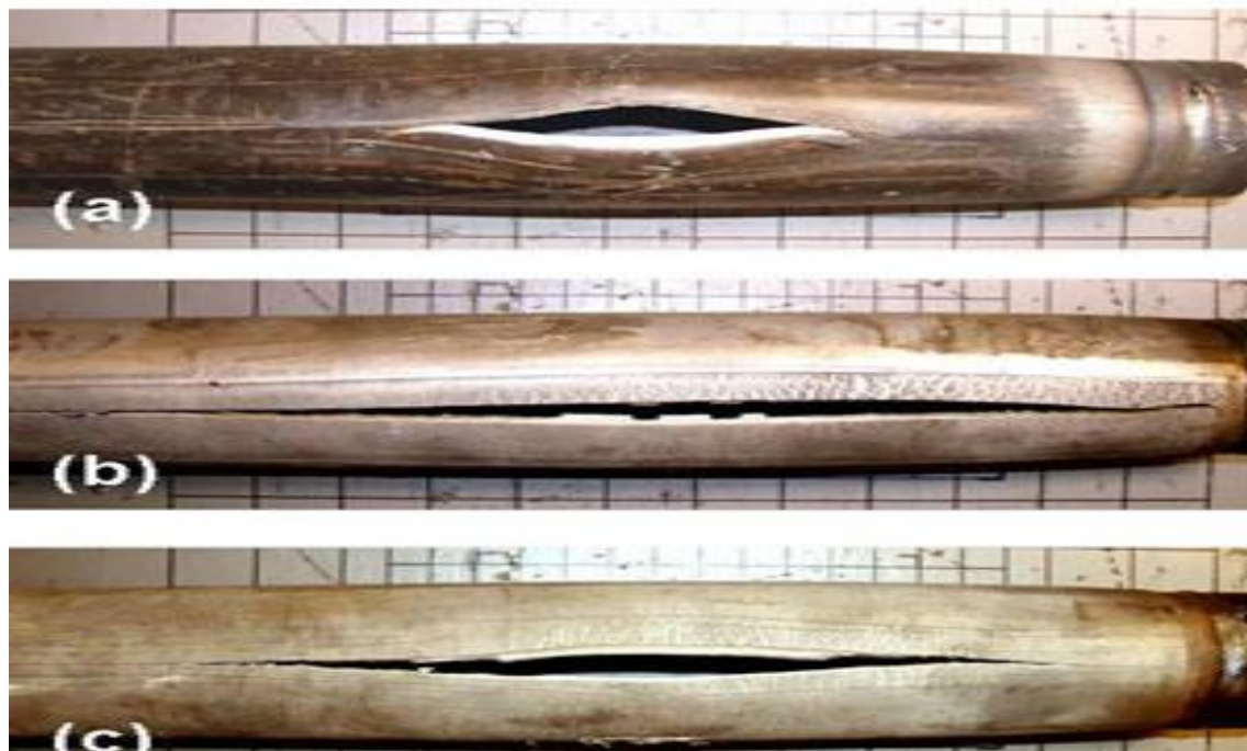
Fig. 4.2 Some of the Damaged Super Heater Tubes.
