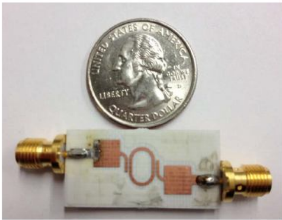
Figure 16: Fabricated elliptical patch resonator bandpass filters
