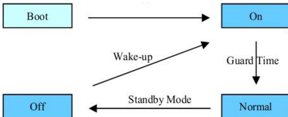
FIG. 4 STATE TRANSITION DIAGRAM OF ELECTRICAL OUTLET
