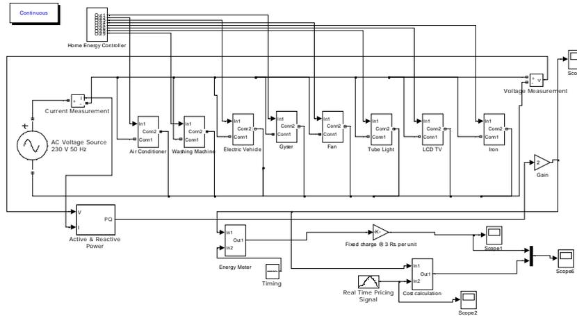
Fig. 5 Simulink Model of Home Area Network.
