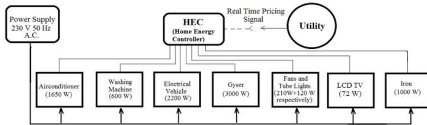
Fig. 4 Block diagram of Home Area Network
