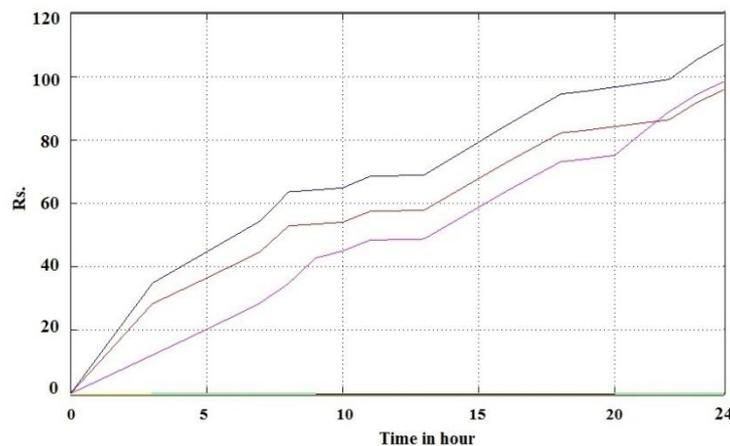
Fig. 9 Cumulative cost of energy consumed. Upper trace: Cost without power scheduling. Middle trace: cost with power scheduling, Lower trace: cost with power scheduling and maintaining load below  $P_{max}$ .
