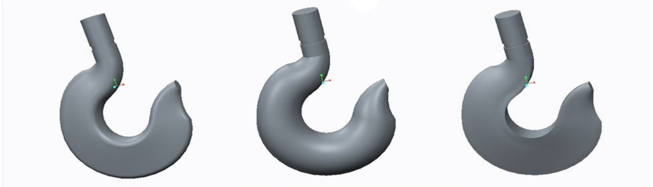
Fig 1 Design of Trapezoidal, Circular and Triangular cross sectioned hook
