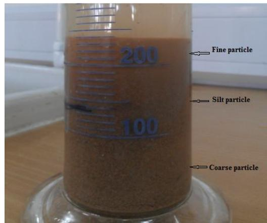
Fig. 2 Sedimentation test
