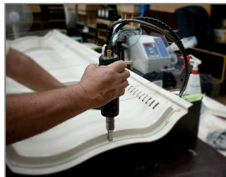
Fig 4 : Ultrasonic spot welding machine and its application
