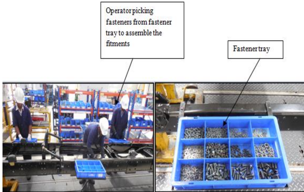
Fig 3 Assembly line (After kaizen)
