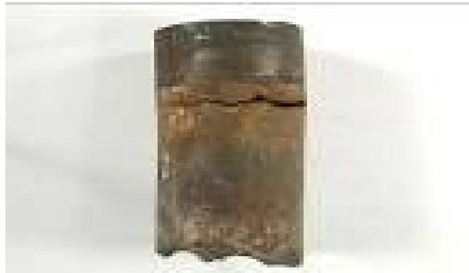
Fig.. 1 Effect of SCC on pipelinehttp (Source: [www.met-tech.com](http://www.met-tech.com))
