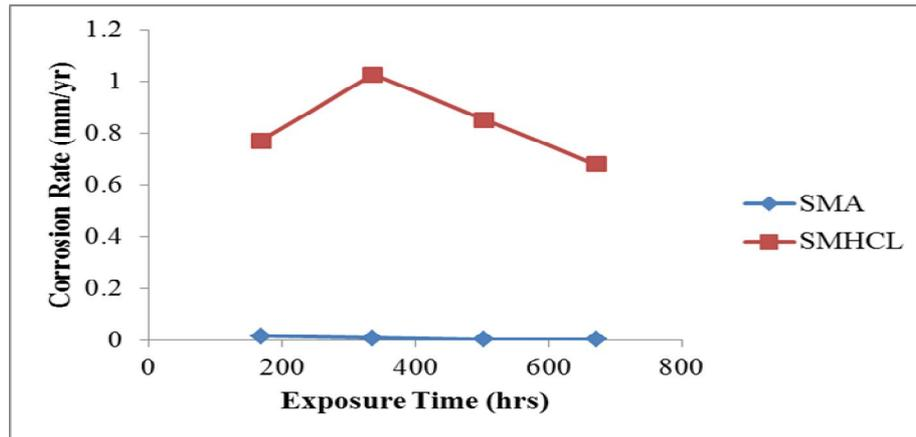
Fig. 6 Corrosion Rates Of Stressed Mild Steel against Exposure Time in Corrosive Media
