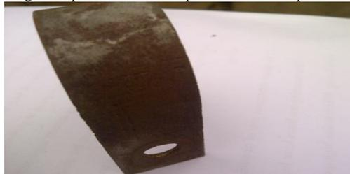
Fig. 3 Corroded U Bend Sample Used in the Experiment
