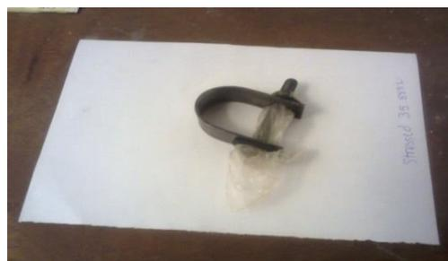
Fig. 2 Prepared U Bend Sample Used in the Experiment
