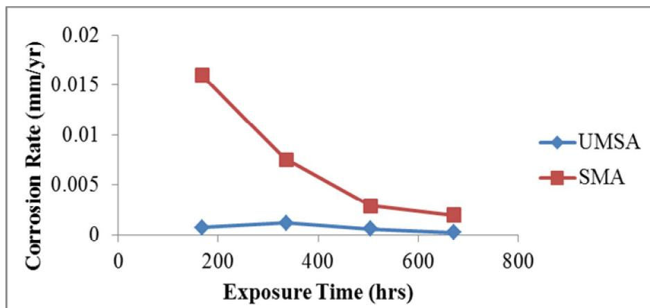
Fig. 5 Effect of Stress on Corrosion Rate of Mild Steel against Exposure Time in Air
