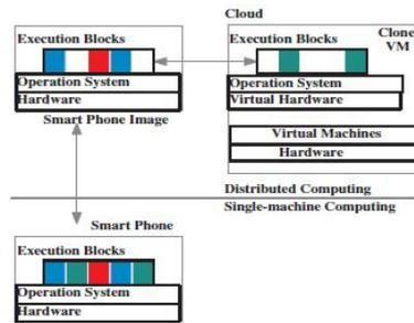
Figure 4: CloneCloud System Architecture
