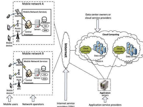
Figure 3: Architecture of Mobile Cloud Computing
