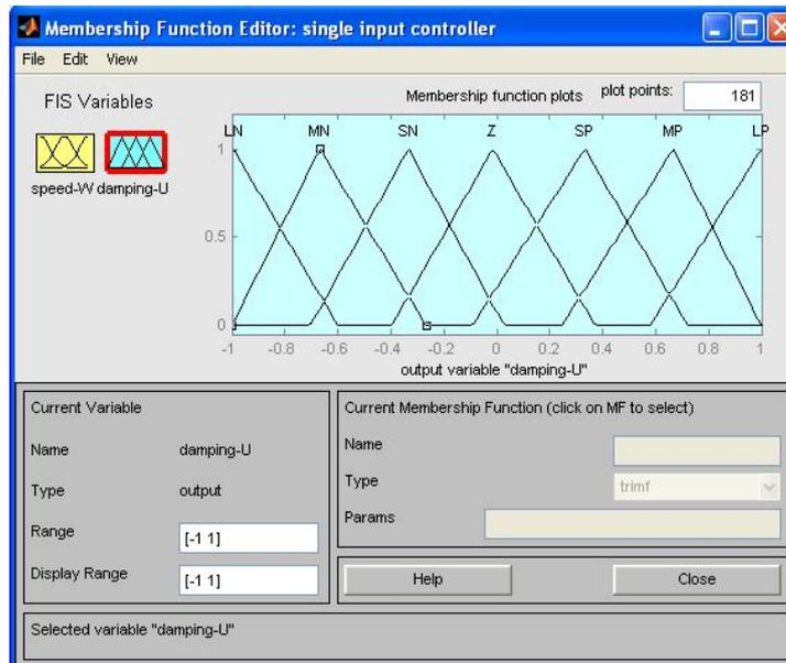
Fig. 4: membership functions for Output  $\Delta u$
