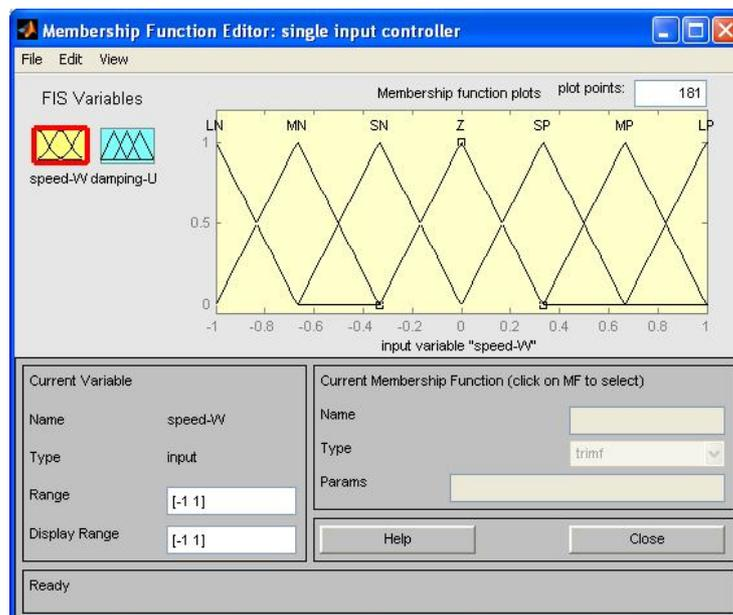
Fig. 3: membership functions for Input  $\Delta\omega$
