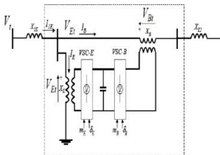
Figure1: UPFC installed in a single-machine infinite-bus power system
