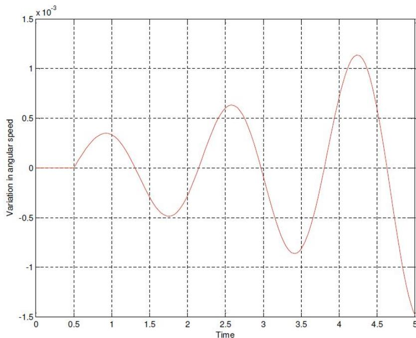
Fig. 5: Response of system without any damping controller
