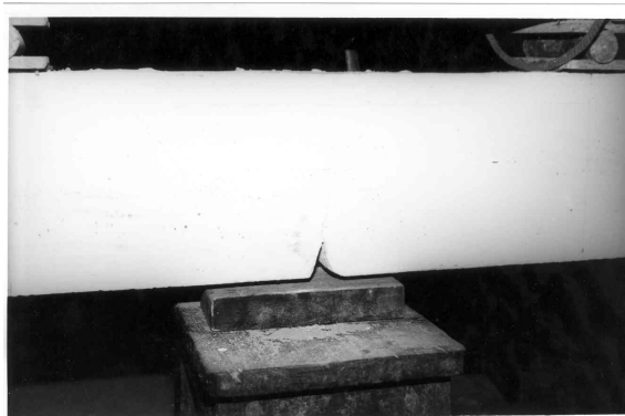
Fig.3. Ferrocement beam with notch
