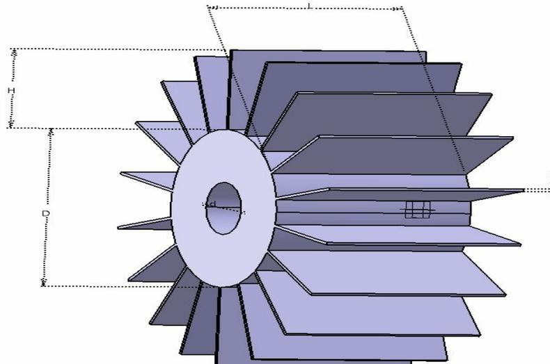
*Fig. 1. Cylindrical heat sink with the longitudinal plate fins.*
