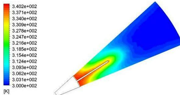
Fig. 4. Temperature contours at  $z = 0.01$  m in  $xy$  plane
