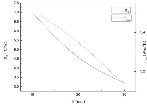
**Fig.5 (b).** The effect of the fin height
