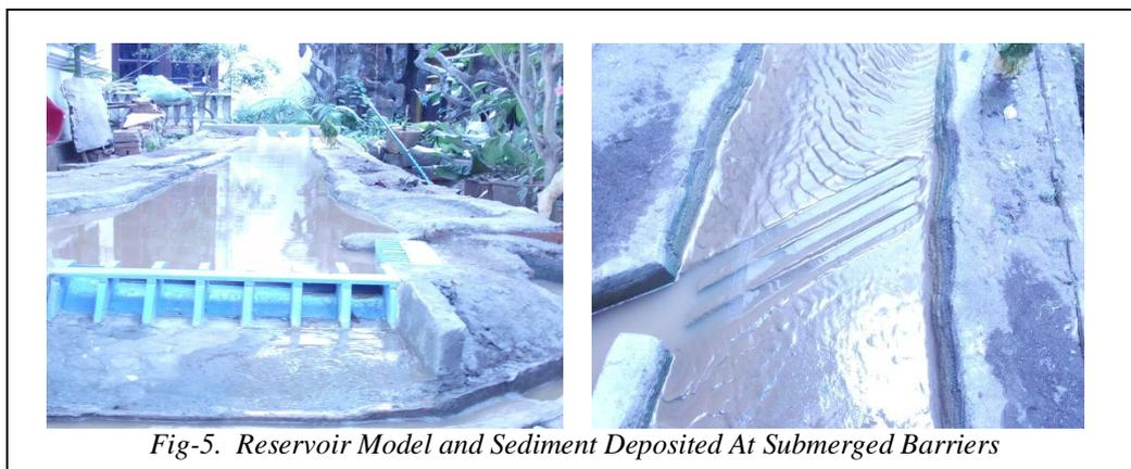
Fig-5. Reservoir Model and Sediment Deposited At Submerged Barriers
