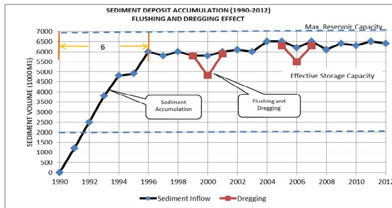
Fig.3. Flushing and Dredging Effect
