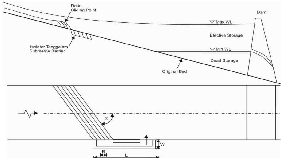
Fig.4. Submerge Barrier Layout
