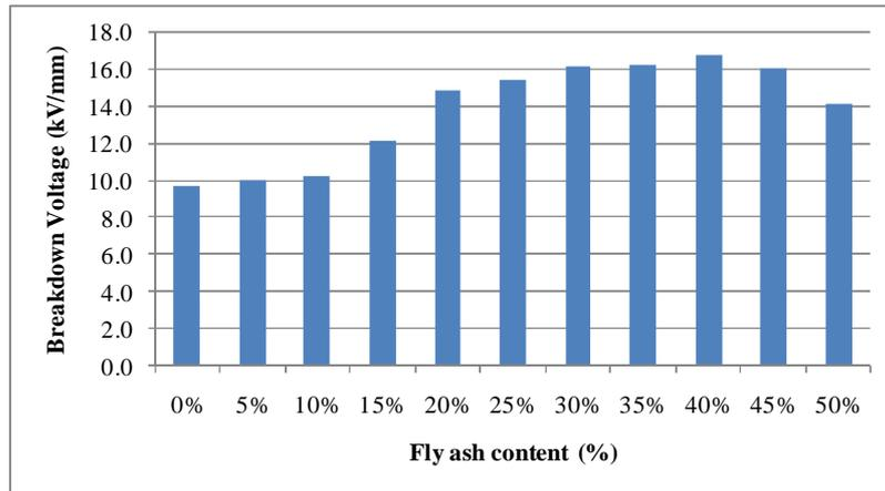
Fig. 4 Effect of fly ash content on dielectric strength of fly ash filled silicone rubber
