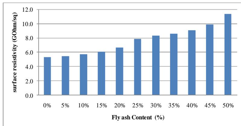
Fig. 6 Effect of fly ash content on surface resistivity of fly ash filled silicone rubber
