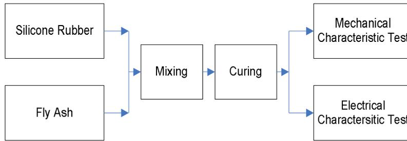
Fig. 1 . Experimental Procedure Flowchart
