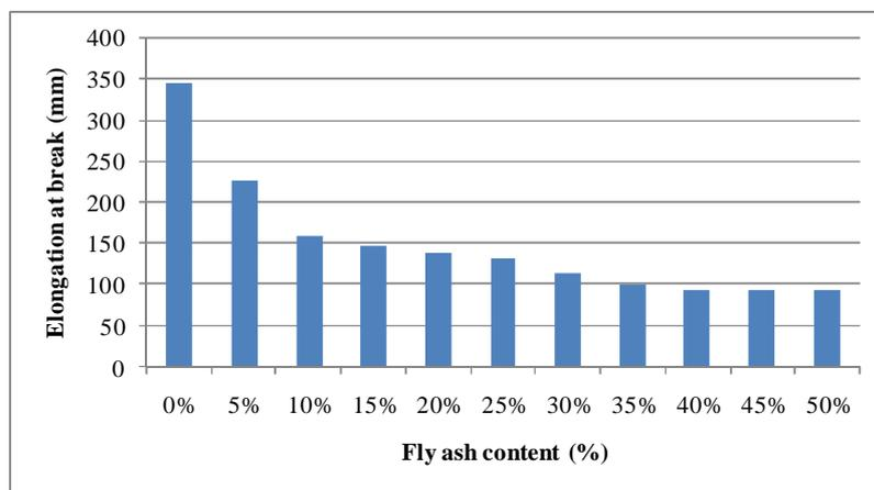
Fig. 3 Effect of fly ash content on elongation at break of fly ash filled silicone rubber
