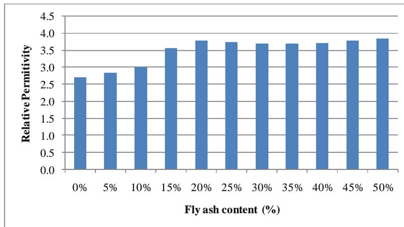
Fig. 5 Effect of fly ash content on relative permittivity of silicone rubber composite
