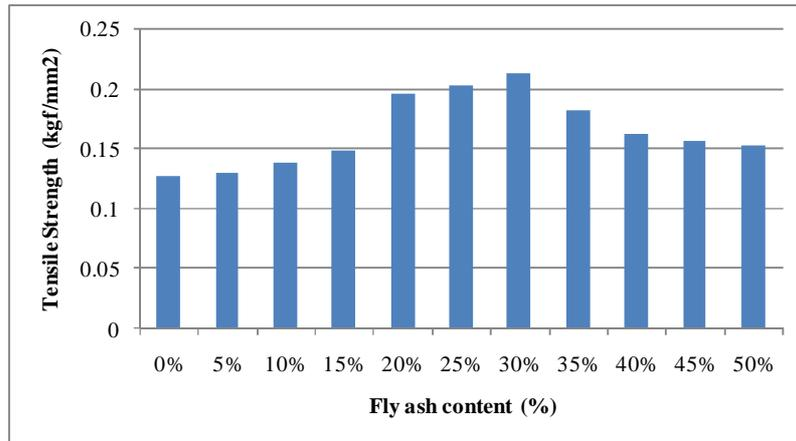
Fig. 2 Effect of fly ash content on tensile strength of fly ash filled silicone rubber
