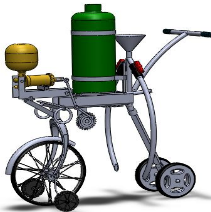
Fig. 1 Chemical sprayer having front wheel has its driver with sprocket and kinematic links
