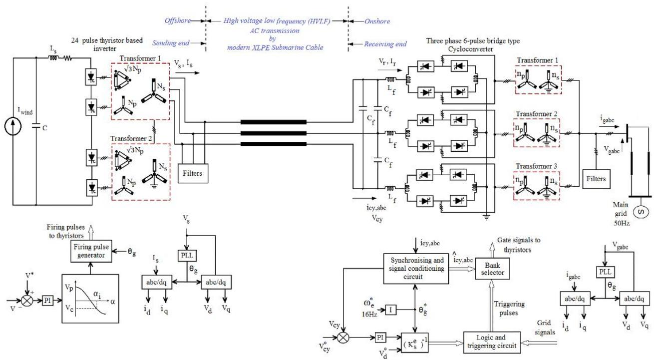
Fig. 1 Test network of Proposed HVLF-AC transmission system for offshore wind power
