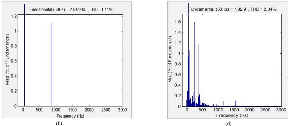
Fig. 4. (a) Voltage wave form at main grid side; (b) FFT analysis for voltage wave form at main grid side; (c) Current wave form at main grid side; (d) FFT analysis for voltage wave form at main grid side.
