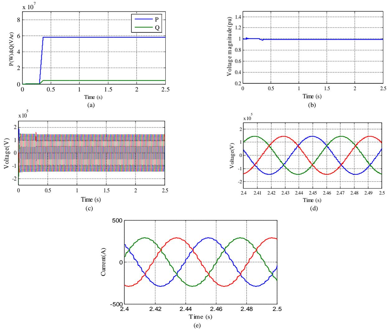
Fig. 3 Waveforms demonstrating the steady-state operation of HVLf-AC transmission system for offshore wind power by modern submarine cable. (a) active and reactive power at receiving end side; (b) voltage magnitude at sending end side transformer (c) voltage waveforms at sending end side transformer; (d). Zooming version of waveform in Fig. 2 (c); (e) current waveform injected into the transmission system.
