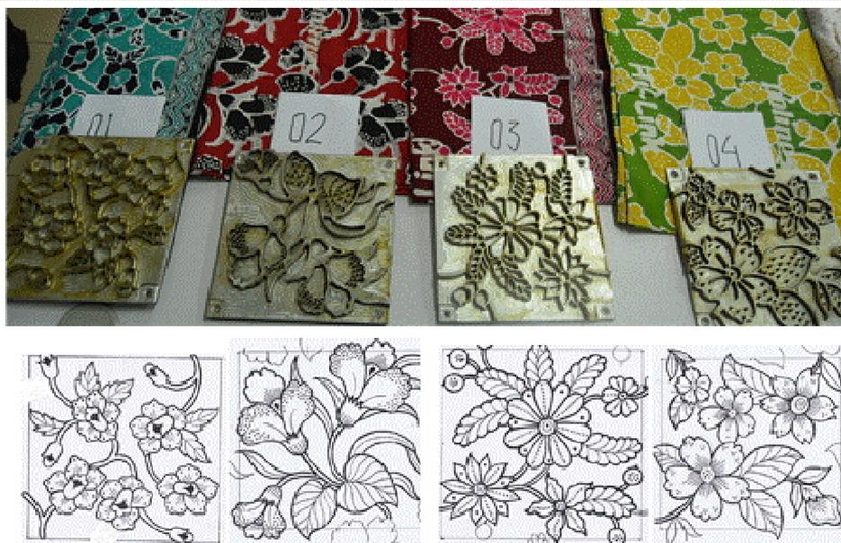
Figure 2. The hand made of batik images (below), the machined batik stamps (middle), and the resulted fabric batiks (top)
