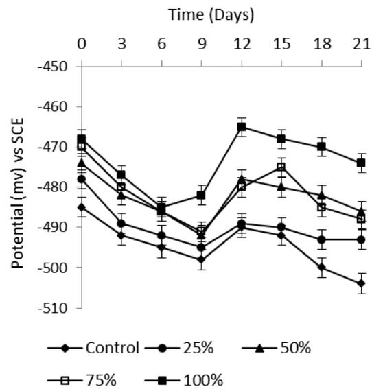
Figure 4: Variation in potential (vs SCE) for mild steel in various concentrations of rosemary extract with passage of time.
