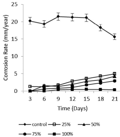
Figure 2: Variation in corrosion rate for mild steel in various concentrations of rosemary extract with passage of time.
