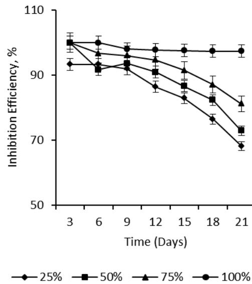
Figure 3: Corrosion inhibition efficiency of various concentrations of rosemary extract with the increase in exposure time for mild steel.
