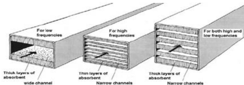
Fig. 2 Absorbing material thickness and baffles spacing example
