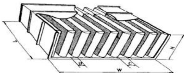
Fig. 1 parallel baffle silencers
