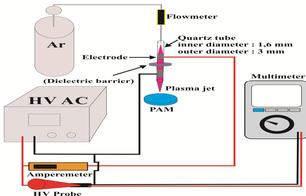
Fig. 1 Schematic of research equipment set-up
