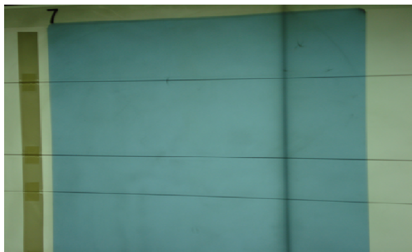
Figure 2: X-ray film of an apron from the CC showing no defects
