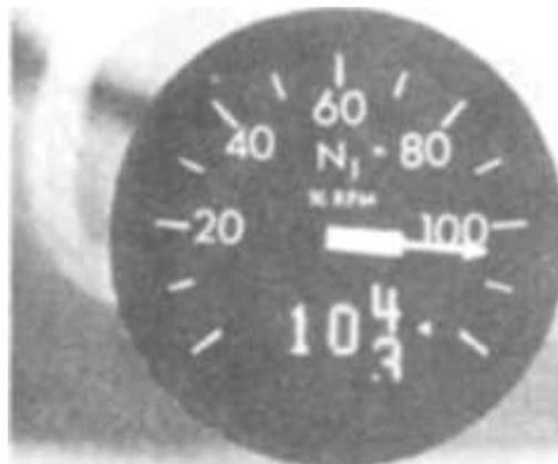
Figure 1.14 Engine speed indicator with a dot matrix LED. (Courtesy of Smith's Industries Ltd.)
