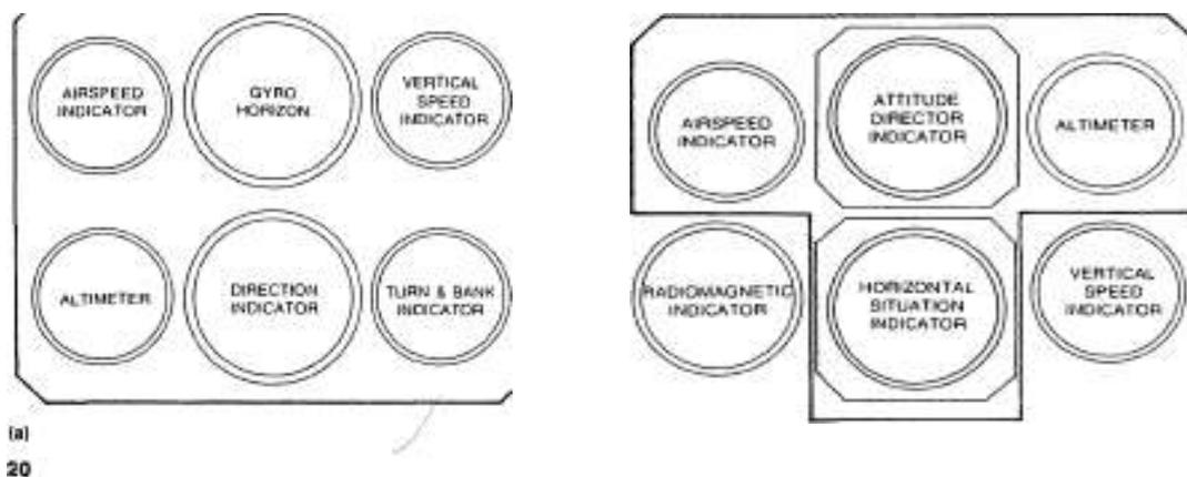
Figure 1.19 Flight instrument grouping, (a) Basic six; (b) basic T (with night director system indicators).
