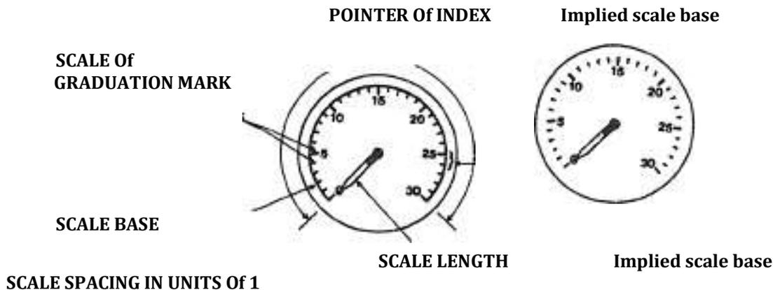
Figure 1.1 Circular scale quantitative display.
