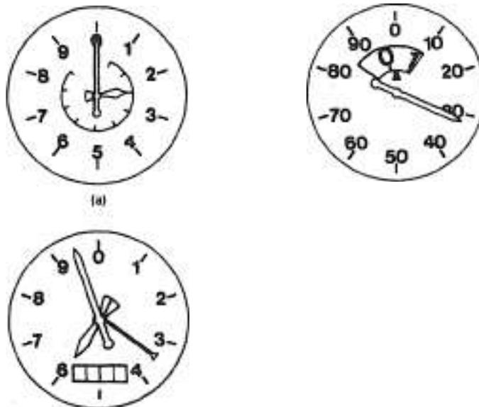
Figure 1.3 High-range long-scale displays, (a) Concentric scales; (b) fixed and rotating scales; (c) common scale and triple pointers.
