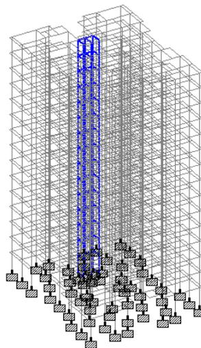
The above given structure is initially modelled for G+14 storey height keeping the same plan dimension. All the Columns were given fixed support at the bottom, which would depict the original foundation in the Building and keep the structure stable. The entire beam ends as fixed as well which would portray the actual condition. For the same structural configuration, modelling of G+7 G+14 and G+21 was performed in both steel and R.C.C.
