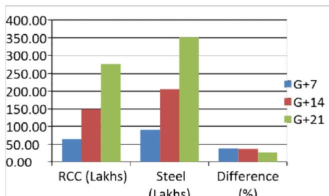
From the statistical results it is obtained that Steel structures are costlier than RCC structures. But it can be seen that as the number of storey increases, the difference between the cost of RCC and steel structures decreases.
