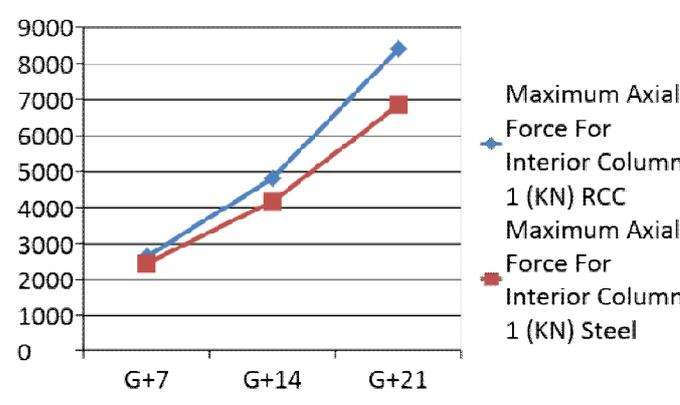
From the above statistical result, it can be concluded that axial force in RCC is much higher than Steel structures. Due to weight of Steel structure is quite low as whereas compared to RCC structure and that will result into higher axial forces in RCC structures.
