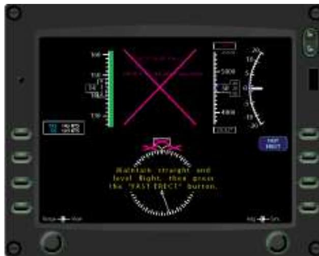
Figure 2-8. A PFD indicating a failed AHRS.
