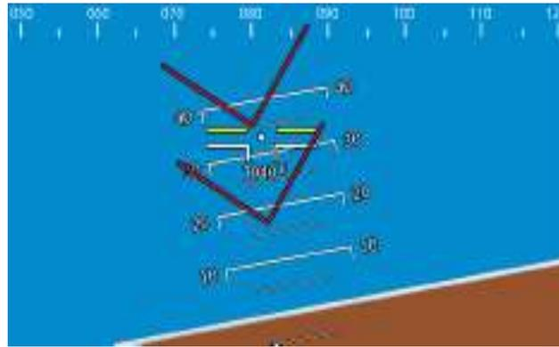
Figure 2-3. Attitude indicator with symbols to assist in recovery from unusual attitude.
