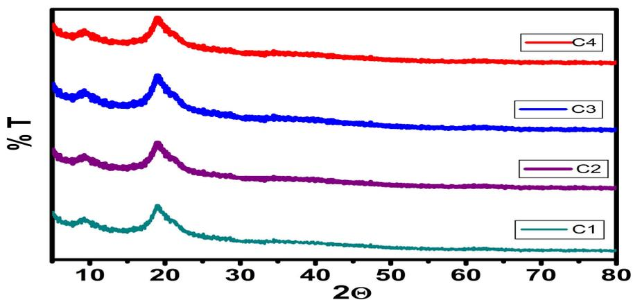
Fig. 1. XRD analysis of Keratin /Chitosan composite nanofibers
