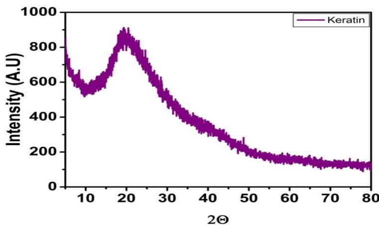
Fig. 4. X-ray diffraction of Keratin
