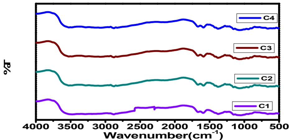
Fig. 5. FTIR spectra of keratin/chitosan composite nanofibers
