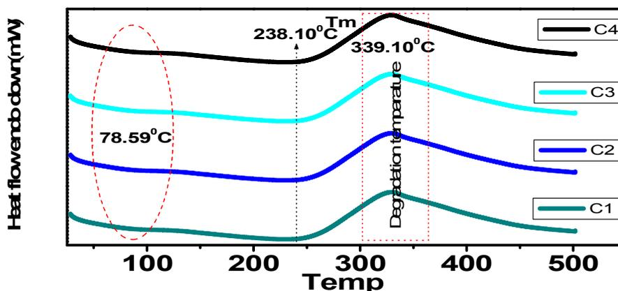
Fig. 7. DSC analysis of keratin/Chitosan composite nanofibers
