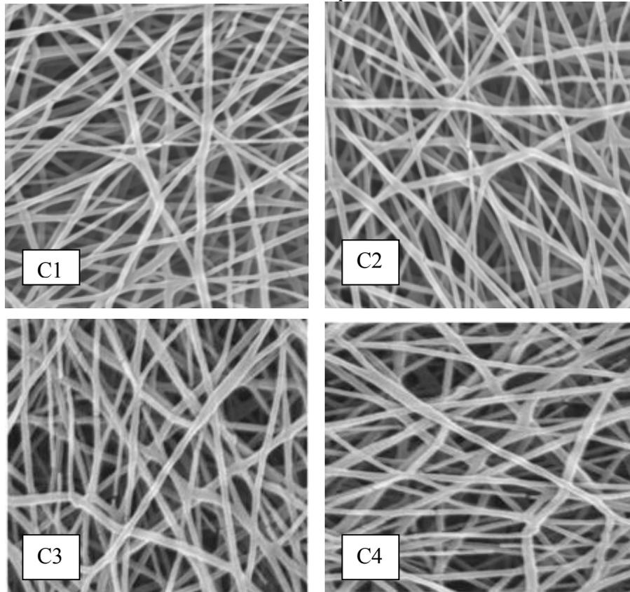
Fig.8. SEM analysis of Chitosan and keratin/Chitosan composite nanofibers
