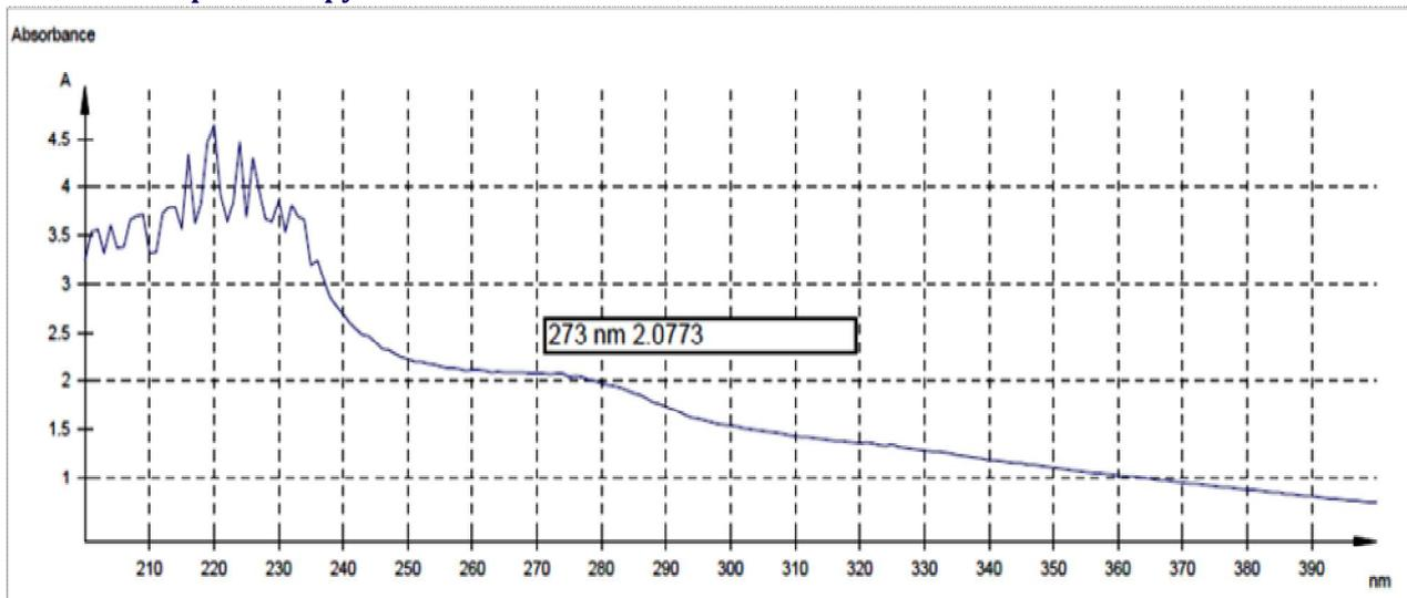
Fig. 1. UV visible spectra of extracted keratin
