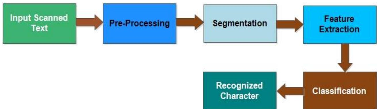
Fig. 3 The components of an OCR system for Proposed System
