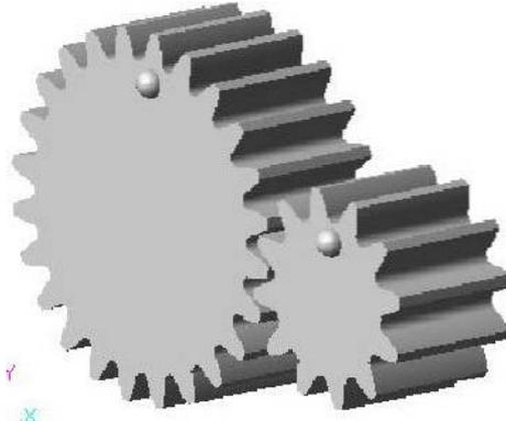
The teeth project radially, and with these "straight-cut gears" Spur gears are gears in the same plane that move opposite of each other because they are meshed together. Gear 'A' is called the 'driver' because this is turned by a motor. As gear 'A' turns it meshes with gear 'B' and it begins to turn as well. Gear 'B' is called the 'driven' gear
