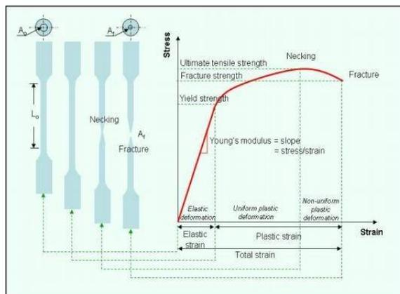
require specific values of spring constants or Young's modulus values. During elastic deformation, the engineering stress-strain relationship follows the Hook's Law and the slope of the curve indicates the Young's modulus (E)
