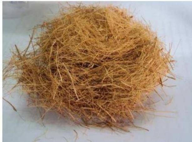
Individual coir fiber has a length of 0.3–1.0 mm, diameter of 0.01–0.02 mm, and aspect ratio of 35. It has medium- to large- sized and polygonal-rounded or elliptic-shaped lumen. The vascular bundle is collateral, which is surrounded by thick sclerenchymatous sheath. Lignin and hemicelluloses that form the cementing materials of fiber cells increase, while the pectin decreases with an increase in the age of the fiber. The fiber becomes stiffer and tougher with
