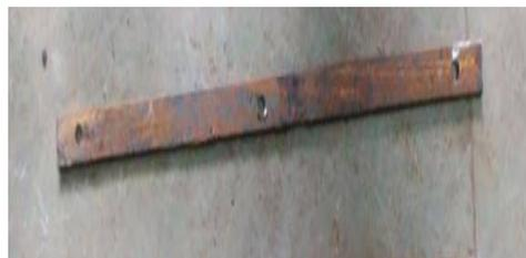
Metal strip is narrow, thin stock that is usually 3/16 in. (4.76 mm) or less in thickness and under 24 in. (609.6 mm) in width. Metal strips are formed to precise thicknesses and/or width requirements.
