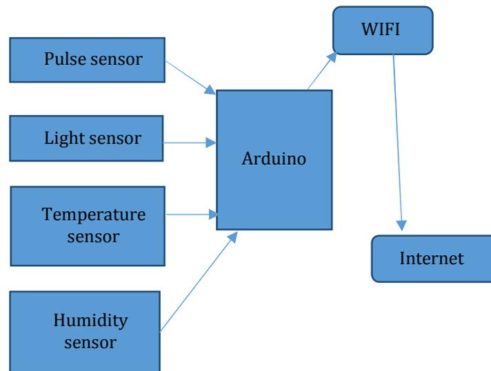
Fig -1.1 - Block diagram
