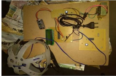
Fig.2.Hardware setup for epilepsy monitoring
