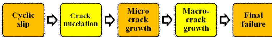
Fig. 1 Phases of fatigue life for nitinol file
