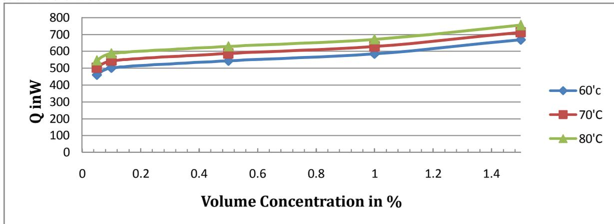
Fig 4: Variation of heat transfer for different volume concentration of CuO Transformer oil nano-fluids for different temperature
