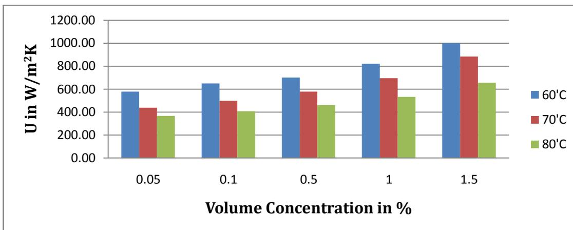
Fig3: Variation of overall heat transfer co-efficient for different volume concentration at different temperature (bar chart)
