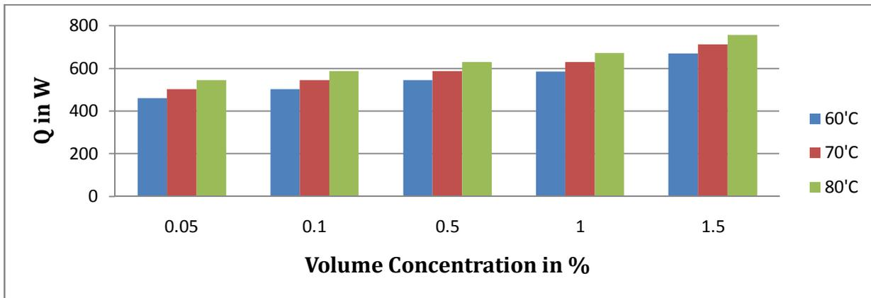
Fig 5: Variation of heat transfer for different volume concentration of CuO Transformer oil nano fluids for different temperature (Bar chart)
