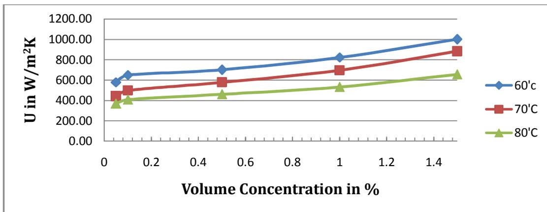
Fig 2: Variation of overall heat transfer co-efficient for different volume concentration at different temperature
