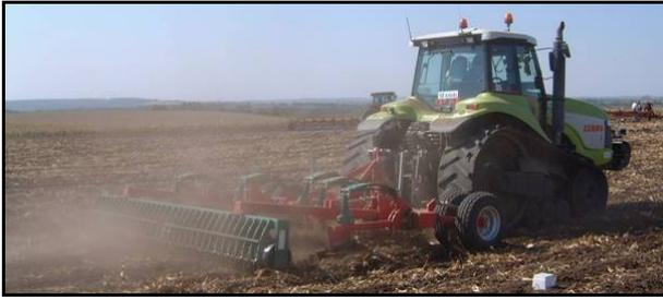
Fig. 3 Kverneland CLE chisel plough
