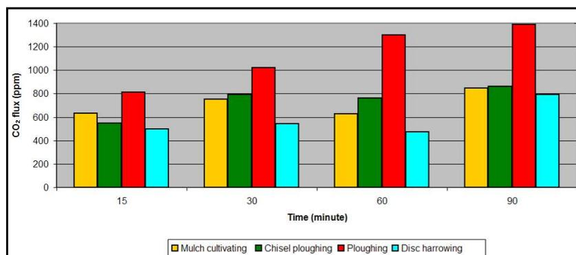
Fig.11: CO<sub>2</sub> flux versus time on different plots
