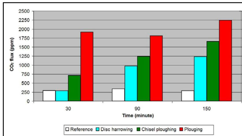
Fig.10: CO<sub>2</sub> flux versus time after different operations
