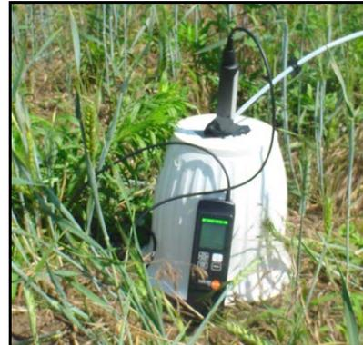
Fig. 7 TESTO 535 CO<sub>2</sub> tester
