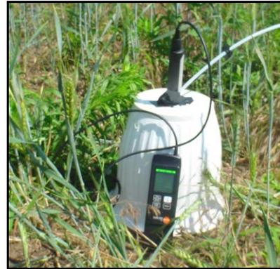
Fig. 7 TESTO 535 CO<sub>2</sub> tester
