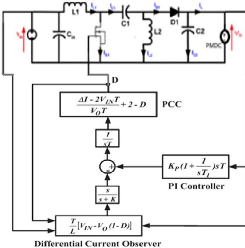
FIGURE 4 Block diagram of SPCC with differential current observer.
