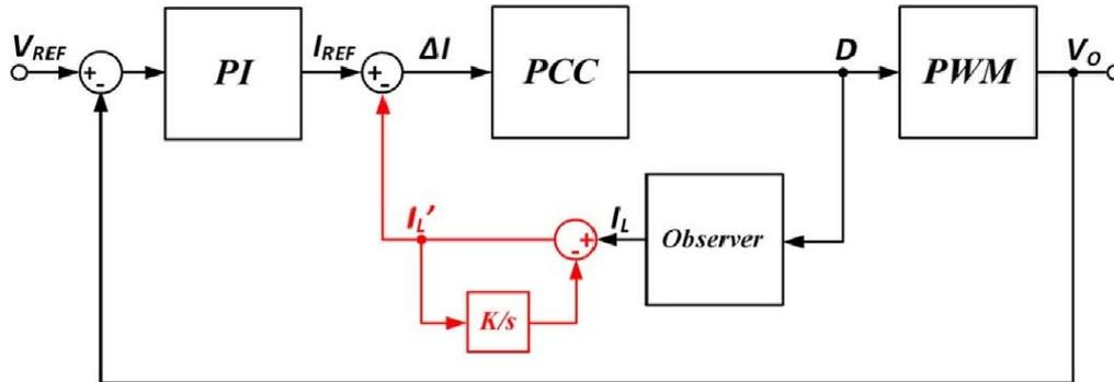
FIGURE 2 Block diagram of the current controller with self-correction
