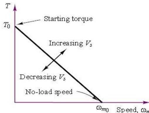
FIGURE 5 Torque speed characteristic of PMDC motor
