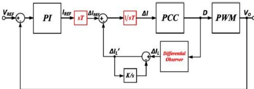
FIGURE 3 Block diagram of the current controller with differential observer
