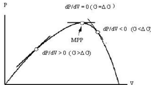
FIGURE 1 PV curve
