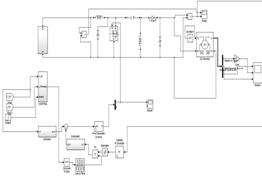
FIGURE 6 Simulink model of sensor less control of PMDC motor
