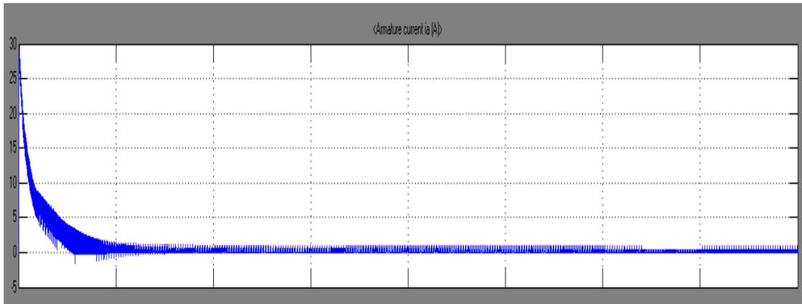
FIGURE 8 Armature current of the PMDC motor
